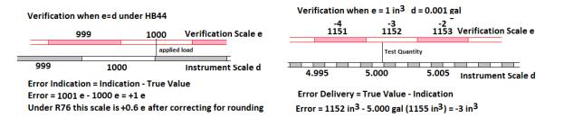
In the above graphics, the instrument scale diverges from the verification scale. They both started at the same zero reference. Notice that the RMFD at right calculates delivery error vs indication error at left. The key is to understand that the verification scale has no error and we are measuring the deviation of the instrument scale from the verification scale.
