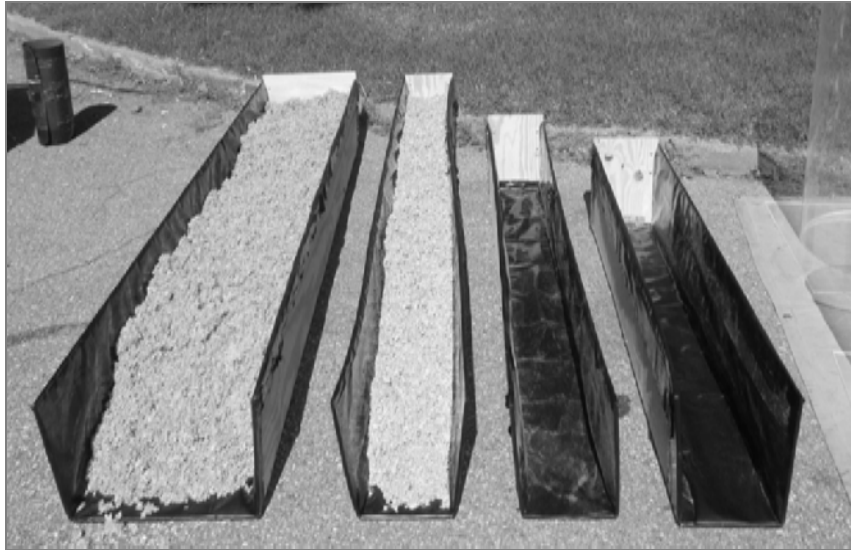
Exhibit 31. The following pictures show how a larger chute (over 280 L) and smaller chutes are used to fill the test measures.
