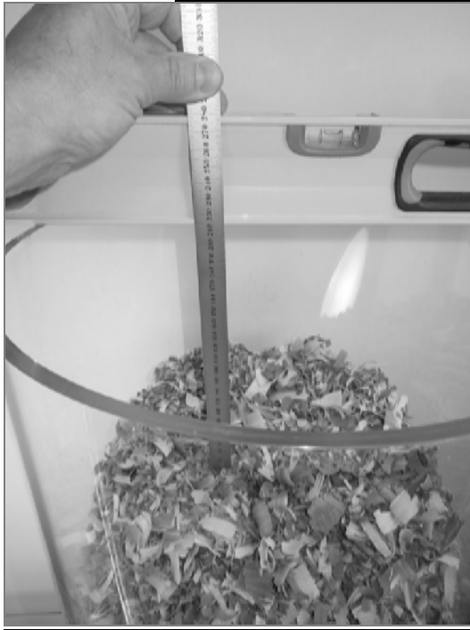
Exhibit 8. Placing ruler into the test measure with zero end down.
