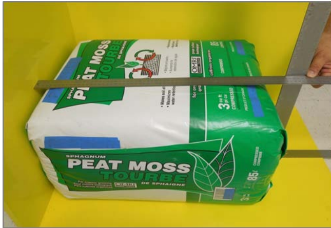
Exhibit 12. Height Measurement – A packaging tail on the end of the package can affect this measurement so it has been folded over and taped against the end of the package.
