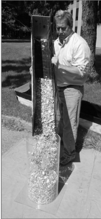
Exhibit 19. Filling a 44 L Test Measure.
