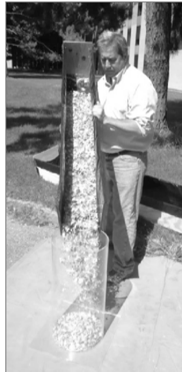
Exhibit 31. The following pictures show how a larger chute (over 280 L) and smaller chutes are used to fill the test measures.
