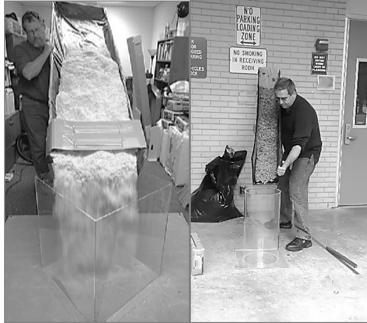
Exhibit 29. Photo to the left shows the use of a chute to pour shredded paper bedding into a 44 L (1.5 cu ft) test measure.
