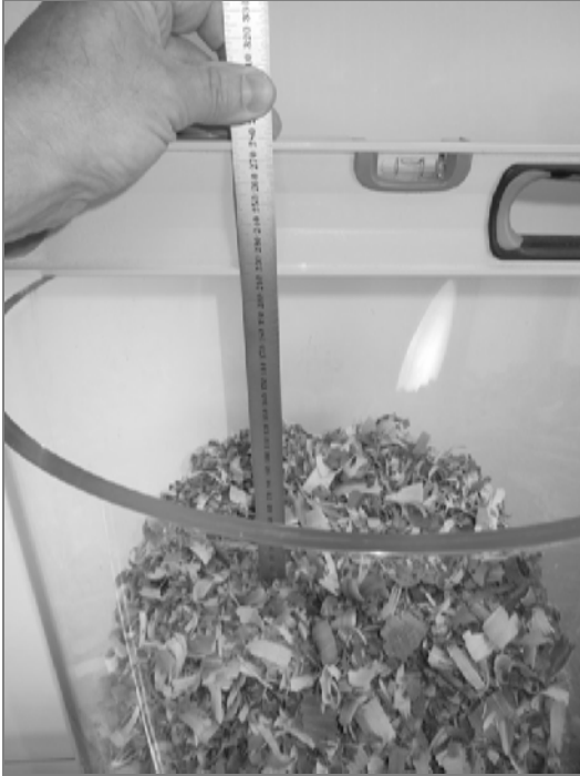
Exhibit 22. Placing ruler into the test measure with zero end down.
