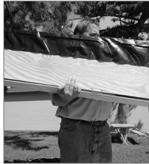
Exhibit 6. Showing how to cradle the chute on one arm and holding it with one hand while tilting it with the other hand.
