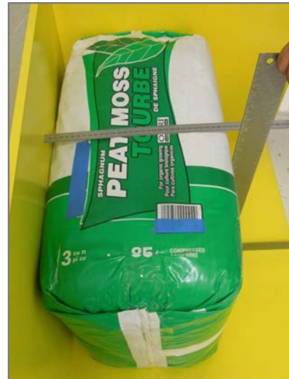
Exhibit 13. Width Measurement – the frame is rotated on its end to vertical so that the carpenter square does not compress the product.
