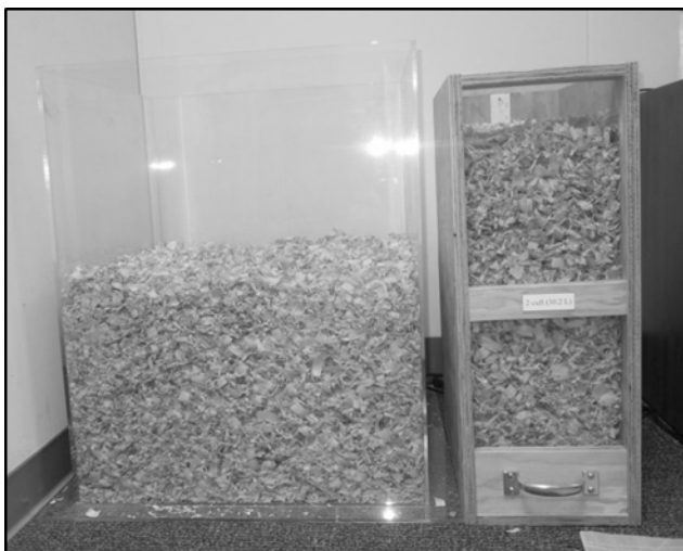
Exhibit 24. Test Measures Used in Study. The large test measures hold up to 279 L (10 cu ft) while the small measures hold up to 52 L (1.5 cu ft).
