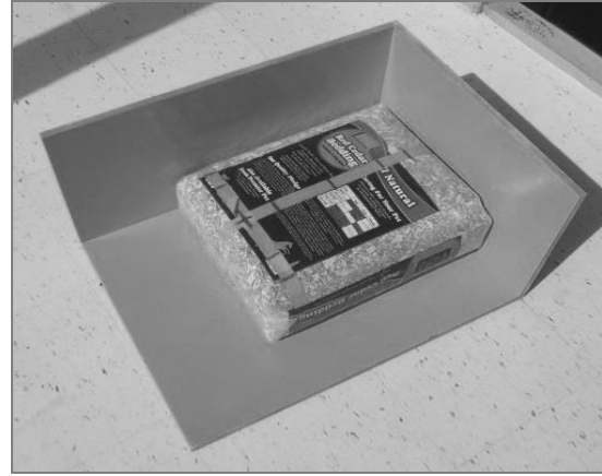
Exhibit 44. Measurement Frame built as an aid to keep reference point stable.
