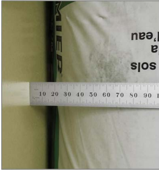
Exhibit 10. The rigid frame allows the observer to hold the zero reference point firmly in place.
