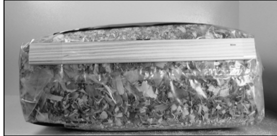
Exhibit 37. Plumped bedding package illustrating rounded edges (angles), which hinders getting accurate measurement points.
