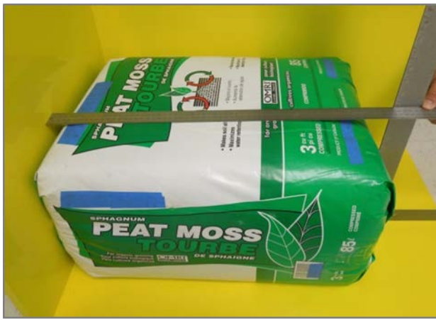
Exhibit 4. Height Measurement – A packaging tail on the end of the package can affect this measurement
