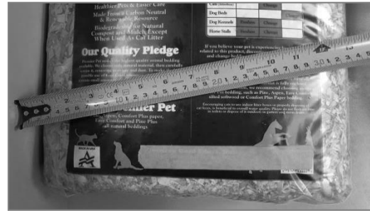
Wrong! Keep the angle of the tape or ruler perpendicular to the edges of the package or trigonometric errors will occur.
