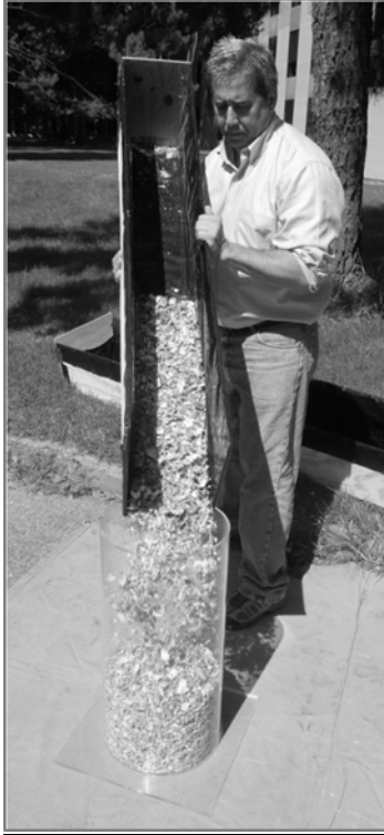
Exhibit 6. Filling a 44 L Test Measure.
