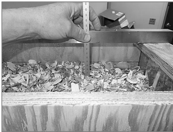
Figure 3. Using the headspace measurement on 56.6 L (2 cu ft) test measure. The ruler is read from the bottom edge of a straight edge or level from a position that reduces parallax.
