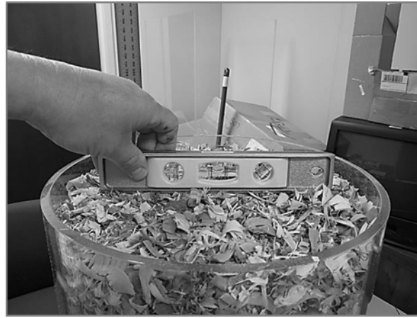
Exhibit 33. Checking Level. Checking the surface of large flake bedding for an approximation of a level condition.
