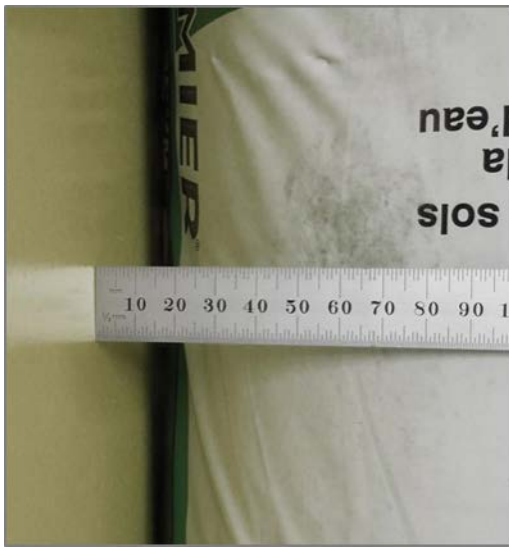
Exhibit 2. The rigid frame allows the observer to hold the zero reference point firmly in place.
