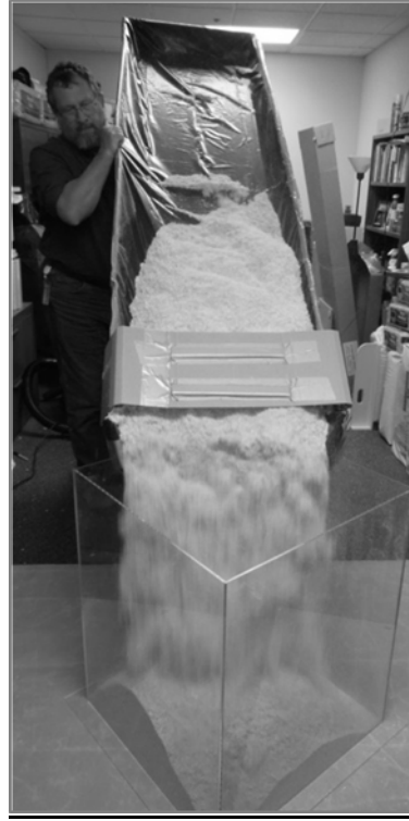
Exhibit 7. Filling a Square Test Measure at an Angle to use the Larger Opening.
