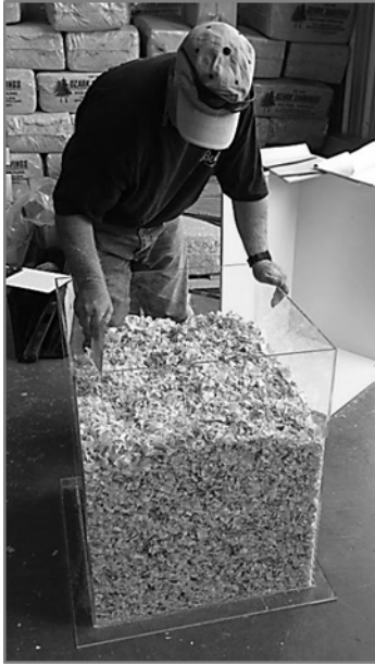
Exhibit 32. Leveling the Surface. Showing the use of a 150 mm mesh to level the surface of large flake bedding.
