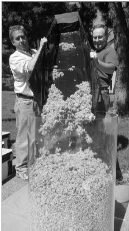
Exhibit 31. The following pictures show how a larger chute (over 280 L) and smaller chutes are used to fill the test measures.
