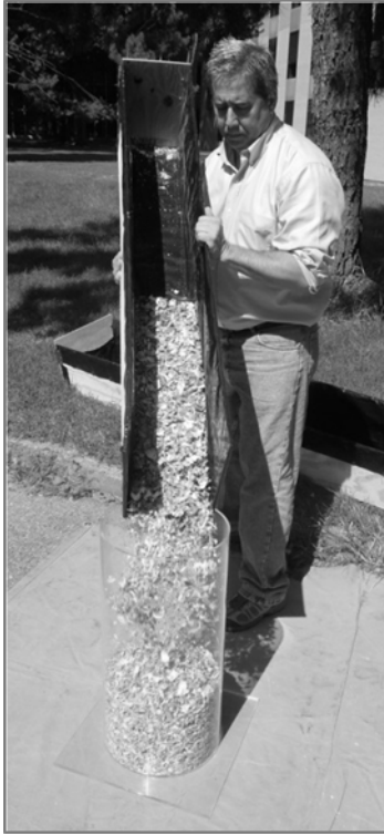
Exhibit 6. Filling a 44 L Test Measure.
