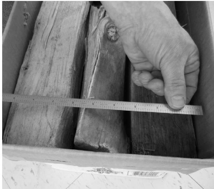
Figure 3.a. – Measuring the Width of the Firewood in a Box
