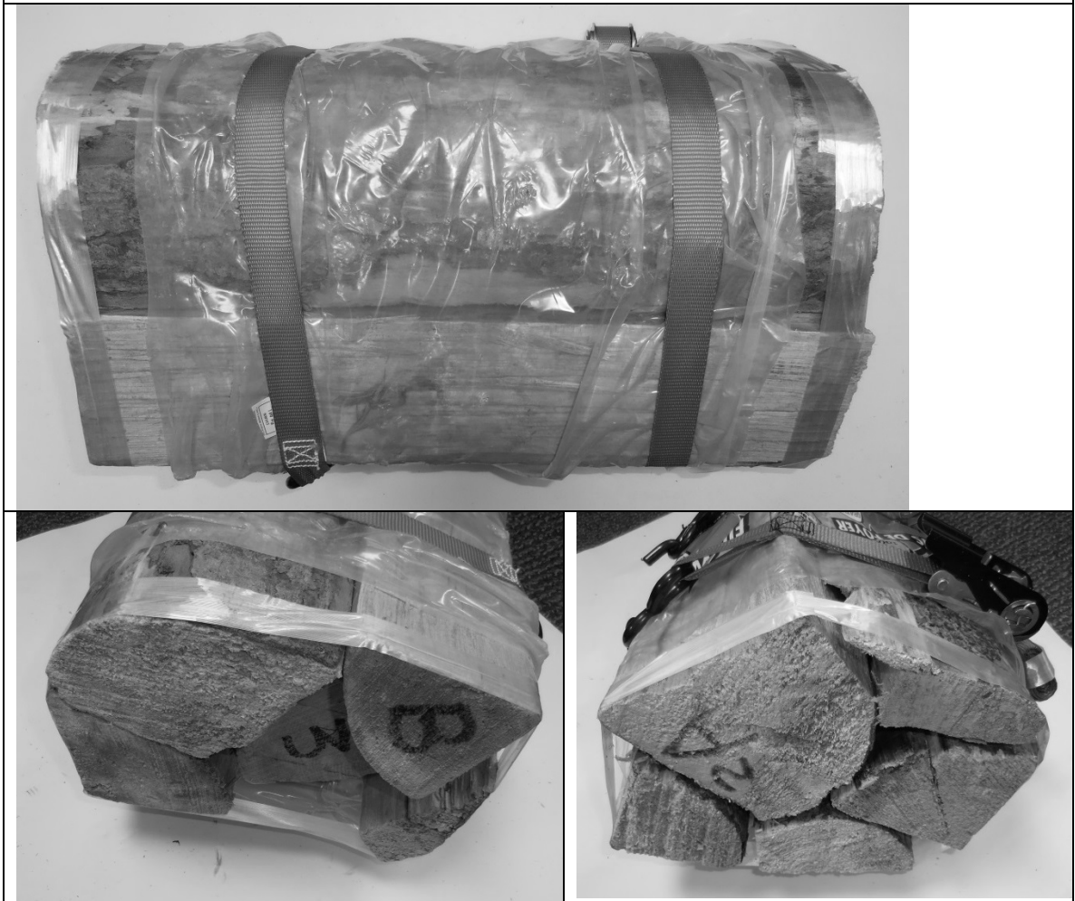
Figure 8. Bundles with Fiber Reinforced Packing Tape around the Perimeter of the Ends
