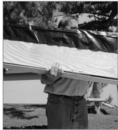
Exhibit 1. Showing how to cradle the chute on one arm and holding it with one hand while tilting it with the other hand.
