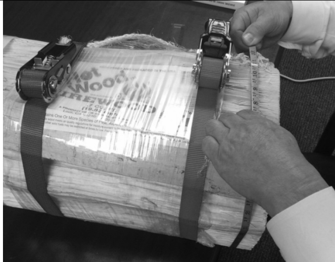
Figure 13. Strapping the End of a Bundle
