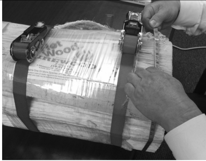
Figure 13. Strapping the End of a Bundle
