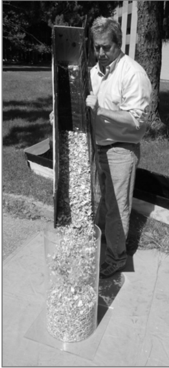
Exhibit 6. Filling a 44 L Test Measure.
