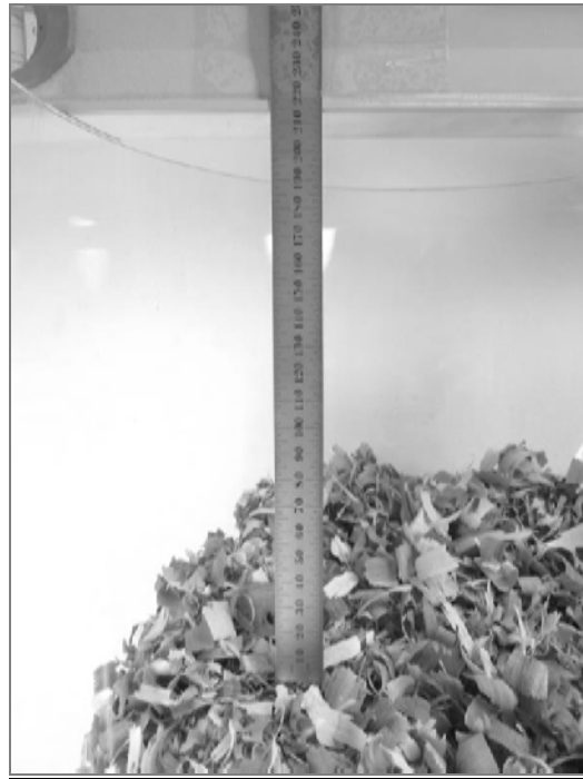
Exhibit 10. Ruler shown with zero end at surface of the bedding.
