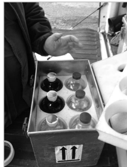
Figure 13b. Sample Box Showing Insulation.
