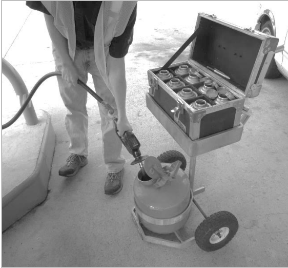
17. Fuel Sampling Cart with Transport Case and Safety Gasoline Can to hold fuel from nozzle-hose flushes.*
