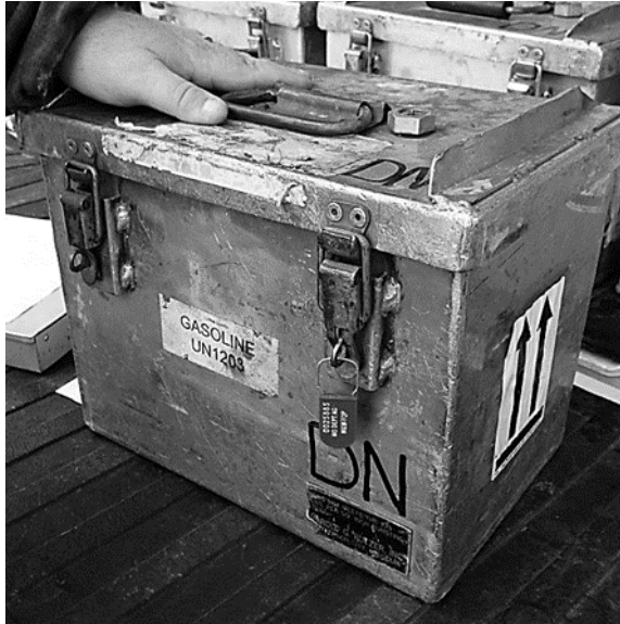
Figure 13c. Sample Box showing Security Seal in Place
