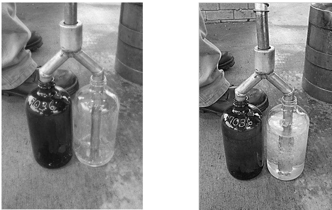
Figure 16. Sample Bottles Empty and Filled with Bifurcated Tube.
