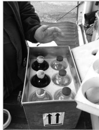
Figure 13b. Sample Box Showing Insulation.
