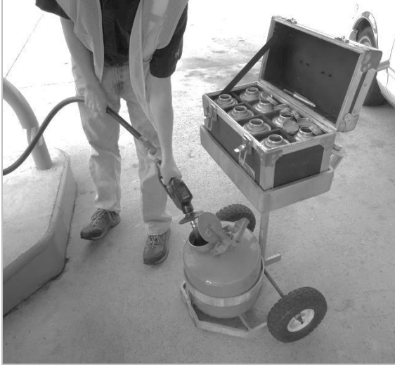
17. Fuel Sampling Cart with Transport Case and Safety Gasoline Can to hold fuel from nozzle-hose flushes.*
