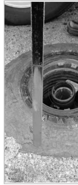
Figure 22. Stick with Paste – No Water Indicated.
